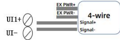
Figure 8: Analog Input Wiring Diagram
